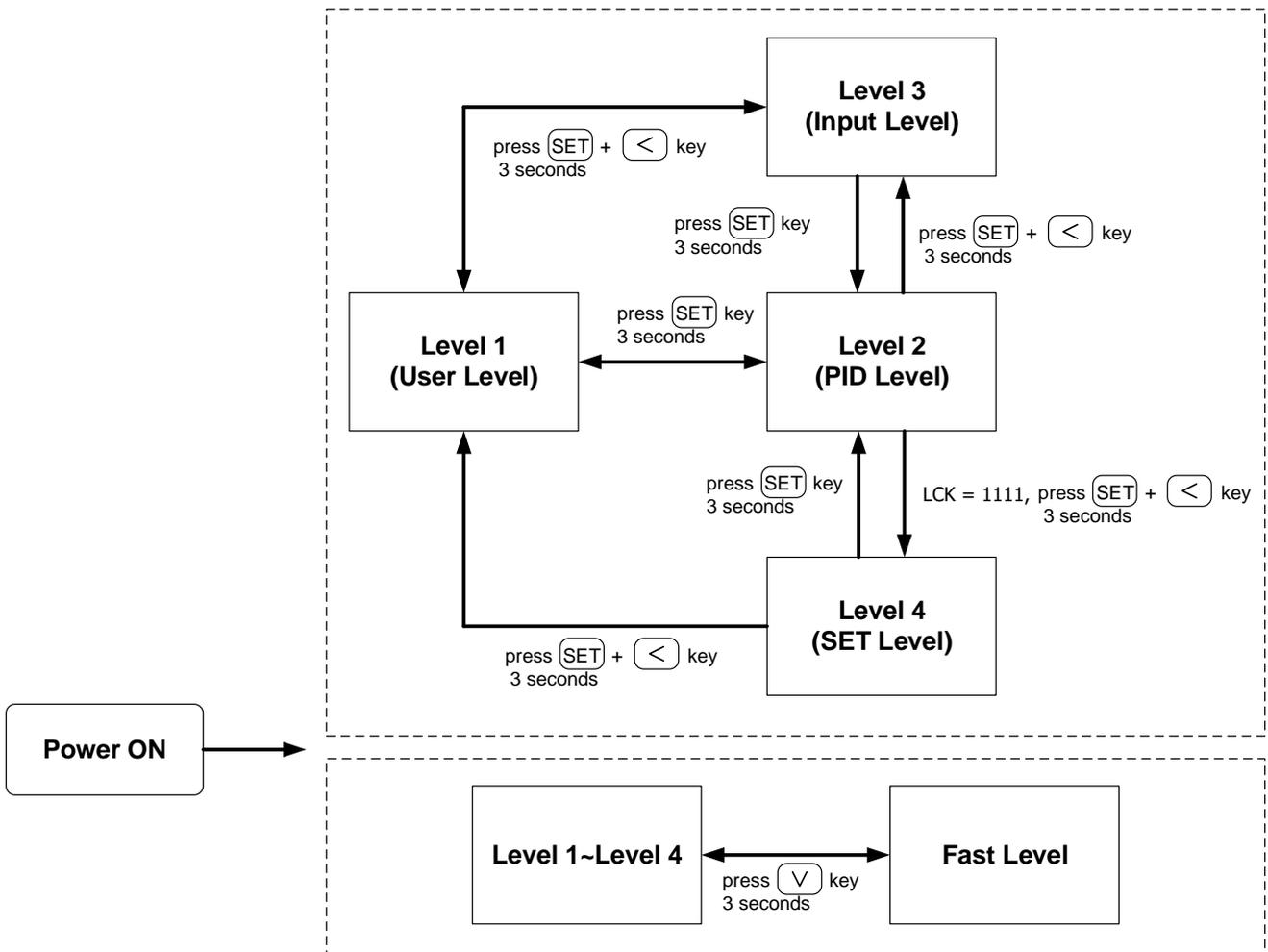
※ : If no key is pressed within 60 seconds, it will automatically return to LEVEL 1 (user level) and display PV/SV.
