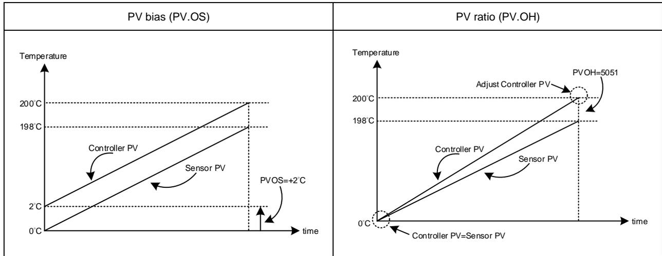
The related parameters of input calibration are as below:
