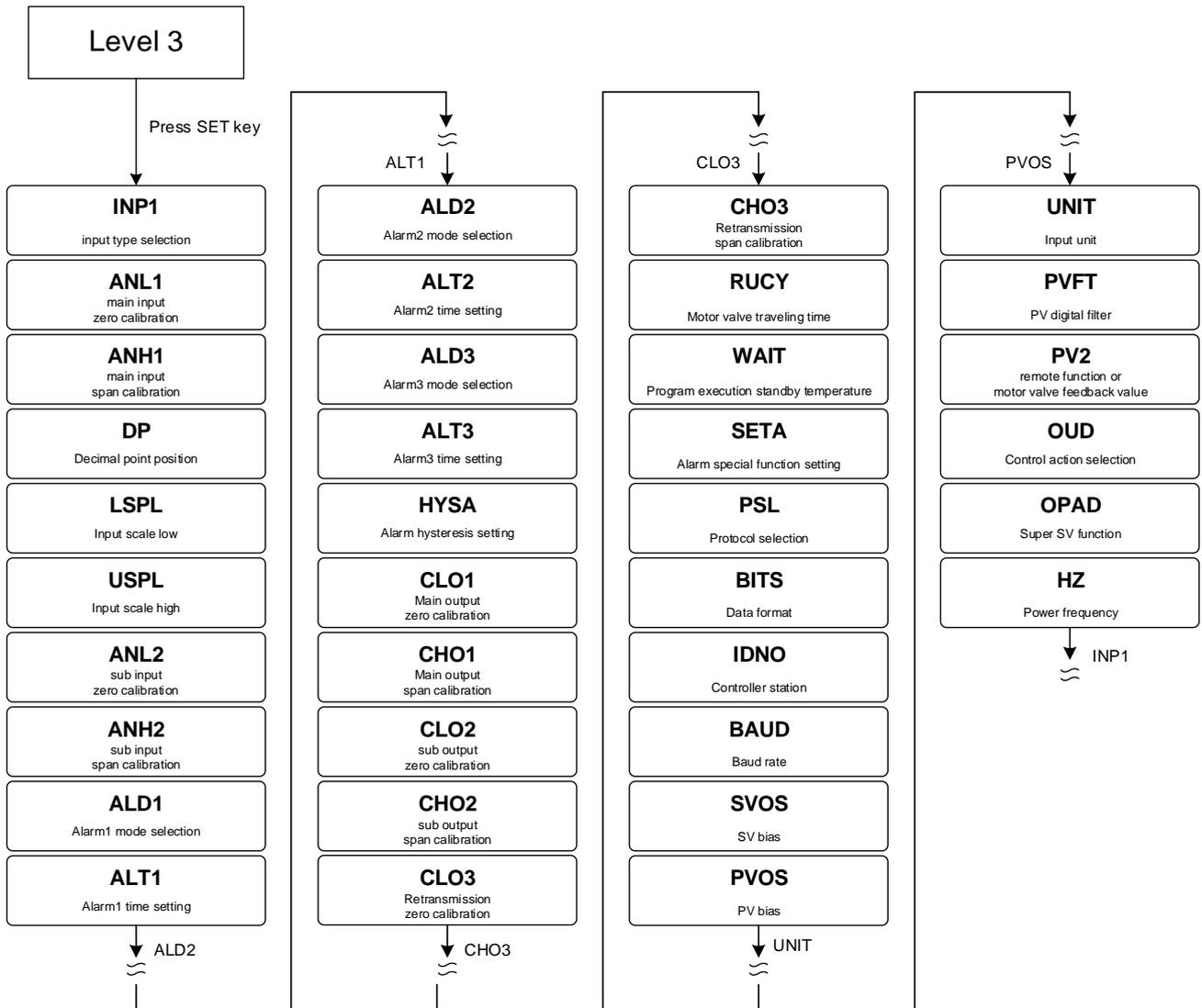
※ If no key is pressed within 60 seconds, it will automatically return to LEVEL 1 (user level) and display PV/SV
