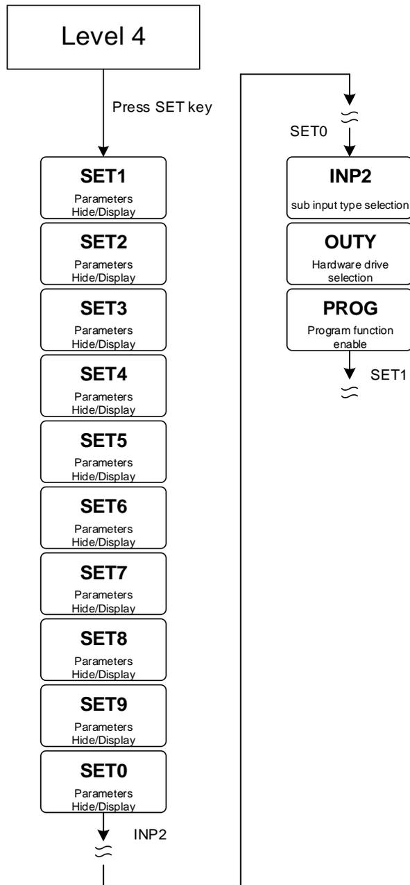
※ If no key is pressed within 60 seconds, it will automatically return to LEVEL 1 (user level) and display PV/SV
