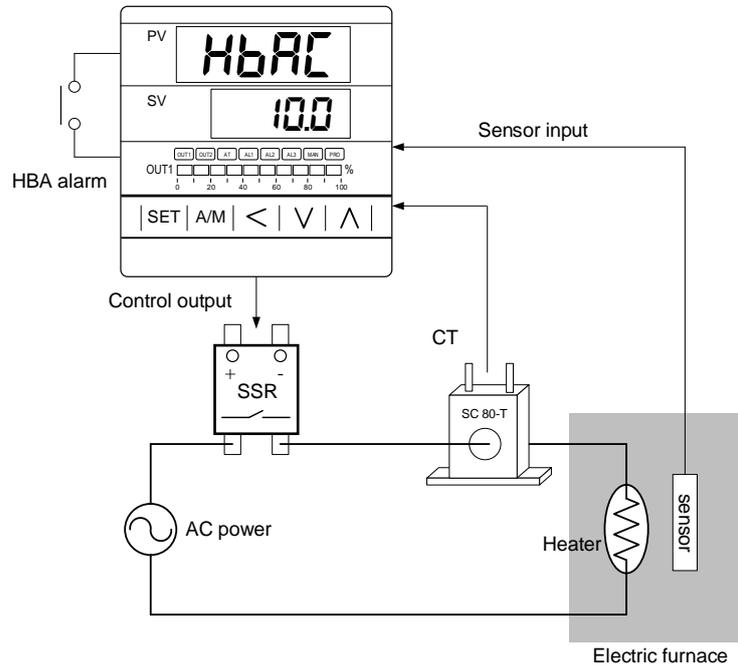
The related parameters of Heater Break Alarm are as below :
