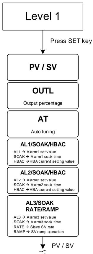
※ : If no key is pressed within 60 seconds, it will automatically return to LEVEL 1 (user level) and display PV/SV
