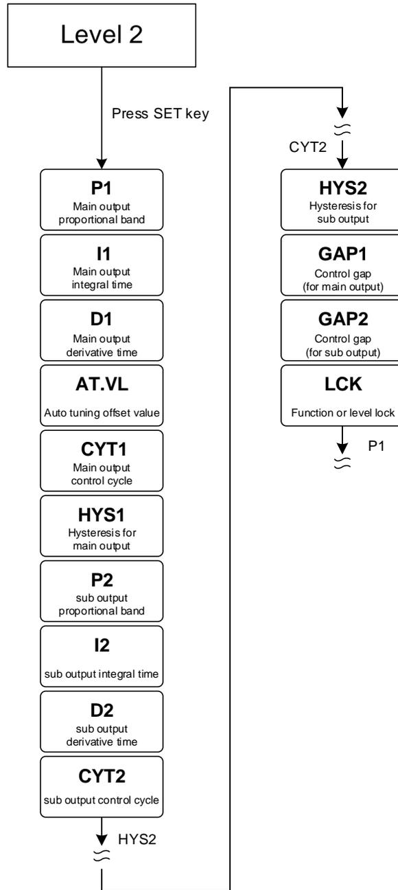
※ If no key is pressed within 60 seconds, it will automatically return to LEVEL 1 (user level) and display PV/SV
